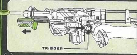
NOTE: Single fire only. You must release the trigger before pulling the SLIDE HANDLE back to avoid jams.
